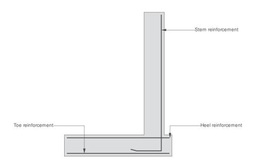
Toe bars - 16 mm dia.@ 200 mm centres -  $(1005 \text{ mm}^2/\text{m})$ The design of the retaining wall heel is beyond the scope of this calculation! Stem bars - 16 mm dia.@ 200 mm centres -  $(1005 \text{ mm}^2/\text{m})$
