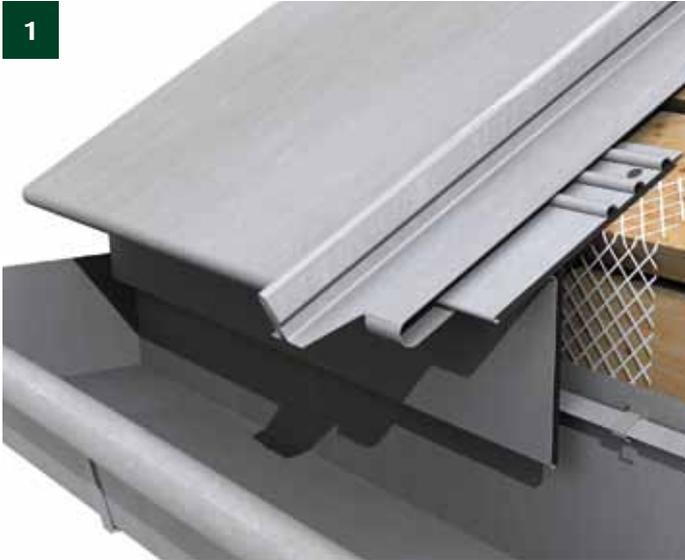
1 Make the nose of the strip in the traditional way: A 30mm fold hooks onto the eaves apron strip G3, so as to make the expansion possible.
