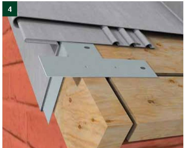
4 For curved roofs (minimum radius of curvature 3 m). Provide a vertical incision in the drip of the verge G3. The incision must be made to one tenth of the value of the radius of the curve (for example: radius of curvature of the roof is 5 m => incision in the verge every 500 mm). For more information please refer contact our services.
