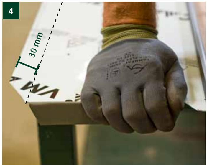
Fold the underside at 180° (height of the fold: 30 mm) across the whole width of the strip and fold the outside across its entire length at 110° (height of the fold: 30 mm).
