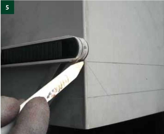
Trace the 'half angle' of the roof. The angle is marked off from the 65 mm line.
