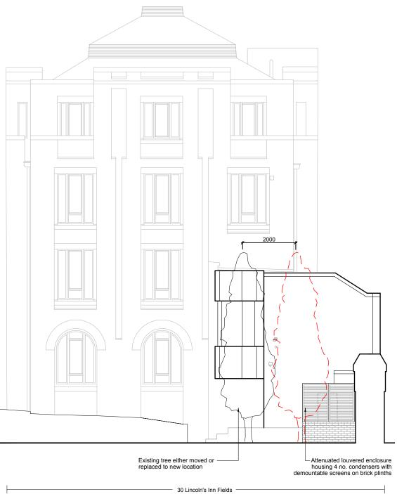
Existing tree either moved or replaced to new location -Attenuated louvered enclosure housing 4 no. condensers with demountable screens on brick plinth W101  $\square$ 1
