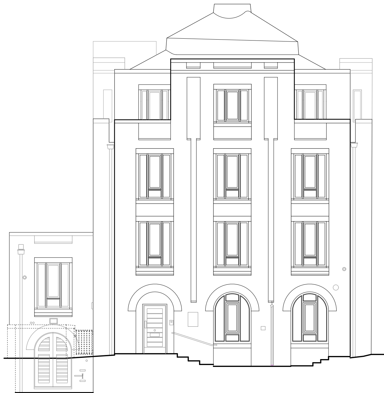
1. Existing NW facing elevation Scale:1/100
