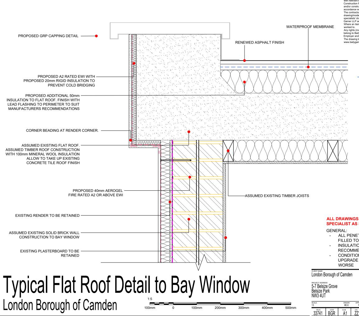
The contractor is responsible for checking dimensions, tolerances, levels and references. This drawing/model is to be read in conjunction with all relevant Other Project Team Members' or specialists' drawings/models/any Federated Model. Any discrepancy is to be notified to Baily Garner LLP and is to be rectified before proceeding with the works on site or shop drawings. Where an item is covered by drawings to different scales, the larger scale drawing is to be
