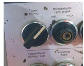
Photo - Inching mode off with gates open while drilling
