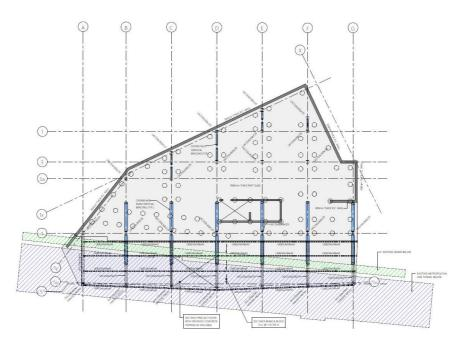
To prevent damage or disturbance to the third-party assets, there are important design considerations which are discussed further below. The Thames Water sewer requires a minimum 1.5m distance between the outside face of the sewer to the outside face of the pile. On this basis the piles will also be outside the 3.0m Tunnel Protection Zone required by LUL.
