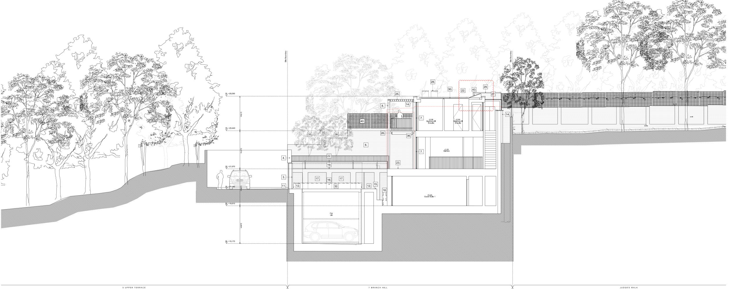
Existing structure / earth New structure Outline of existing house Legend, Proposed Building New 'Bronze' (Electroplated Aluminium) front door New 'Bronze' (Electroplated Aluminium) fixed panels New 'Bronze' (Electroplated Aluminium) sliding gate New brickwork retaining wall in stock brickwork re-claimed from demolition
