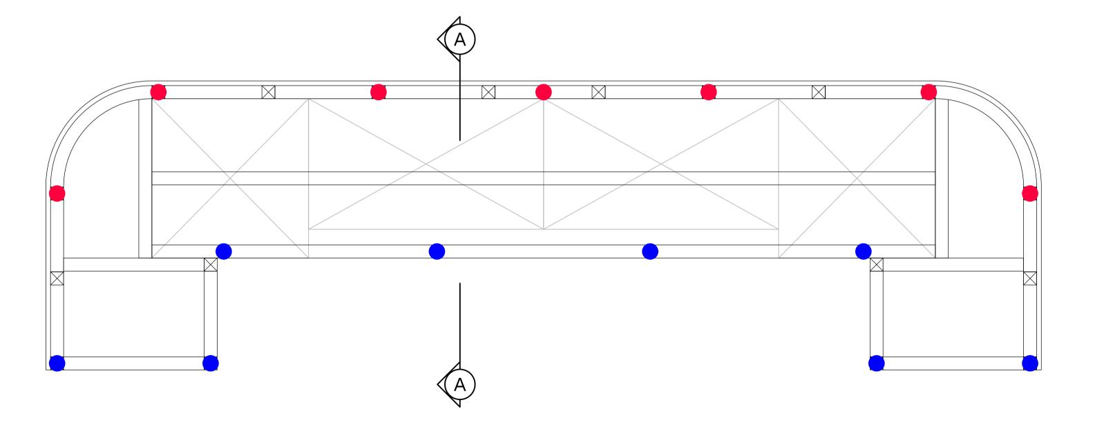
PROPOSED PLAN ON MOVEABLE BAR SHOWING CASTOR WHEEL POSITIONS SCALE 1:10 AT A1
