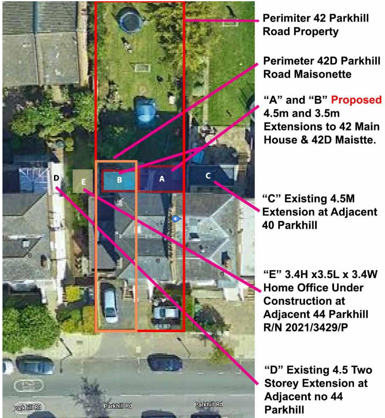
Fig 4 : Plan view of proposed “A” and “B” extensions in context of existing extensions “C”, “D” and home office “E” at adjacent nos 40 and 44 Parkhill Road
