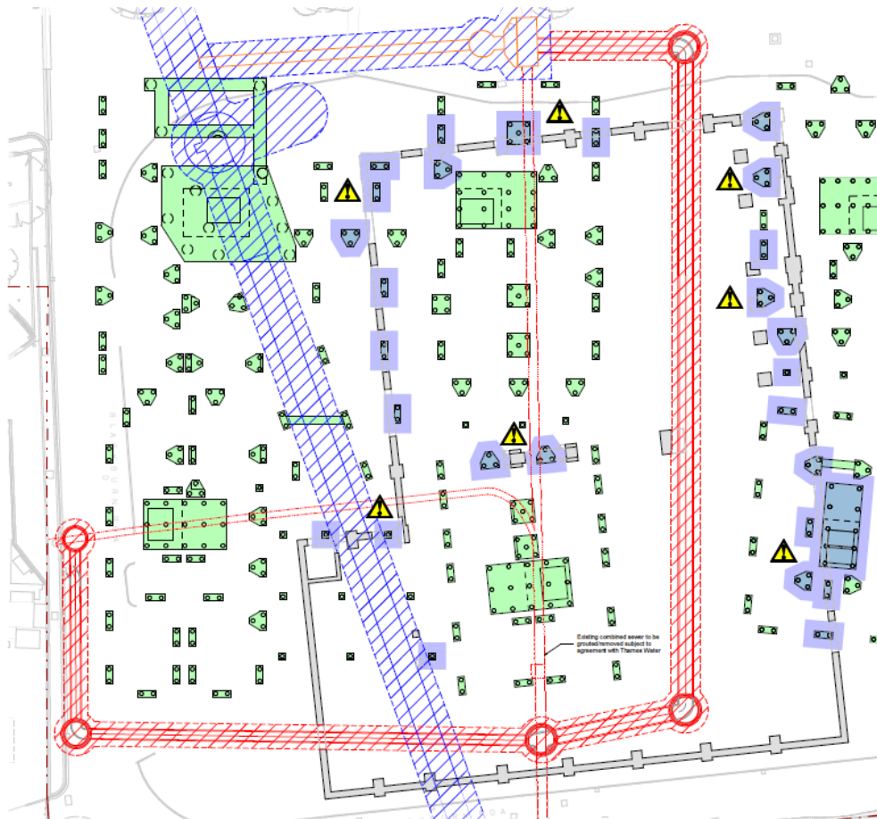
Figure 7 Homebase foundations (grey) and foundations of the new building (green and purple).
