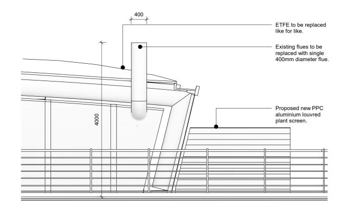
Bloomsbury Place Existing Elevation - Generator Flue
