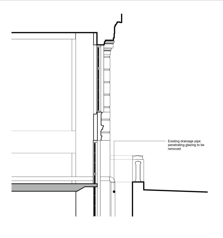
New louvres serving the liquid nitrogen store proposed to be installed behind existing window frame to match existing. Existing stone facade unaltered Liquid Nitrogen store New louvres serving the basement level at B1 proposed to be installed behind existing window frame to match
