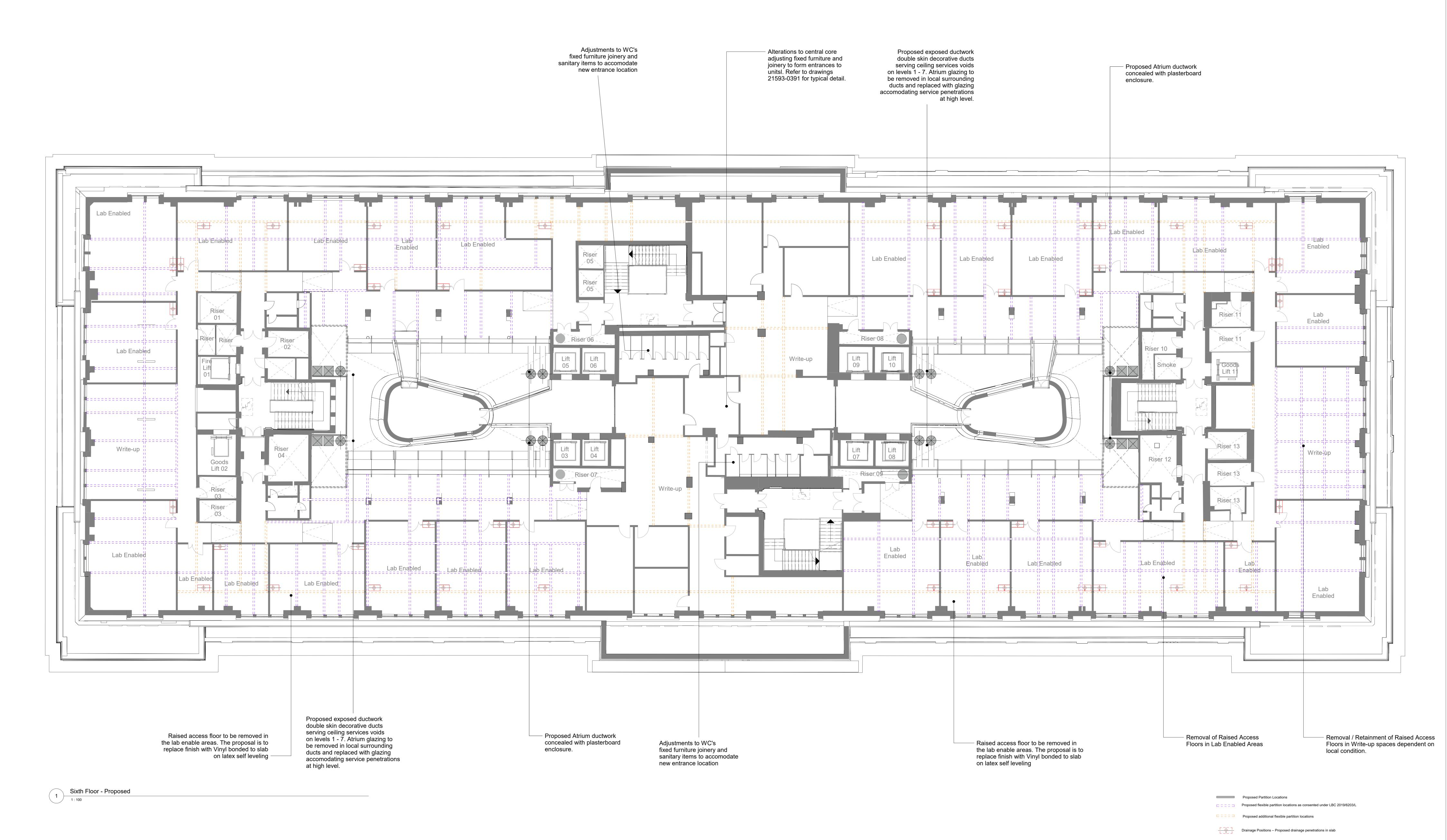
Ramps – Proposed 'illustrative' location of transition in level from slab to raised access floor. Location dependent on final tenant fit out.
