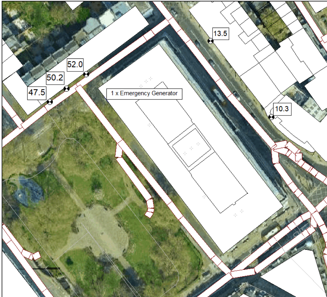
Figure 11 Daytime assessment of emergency generator
