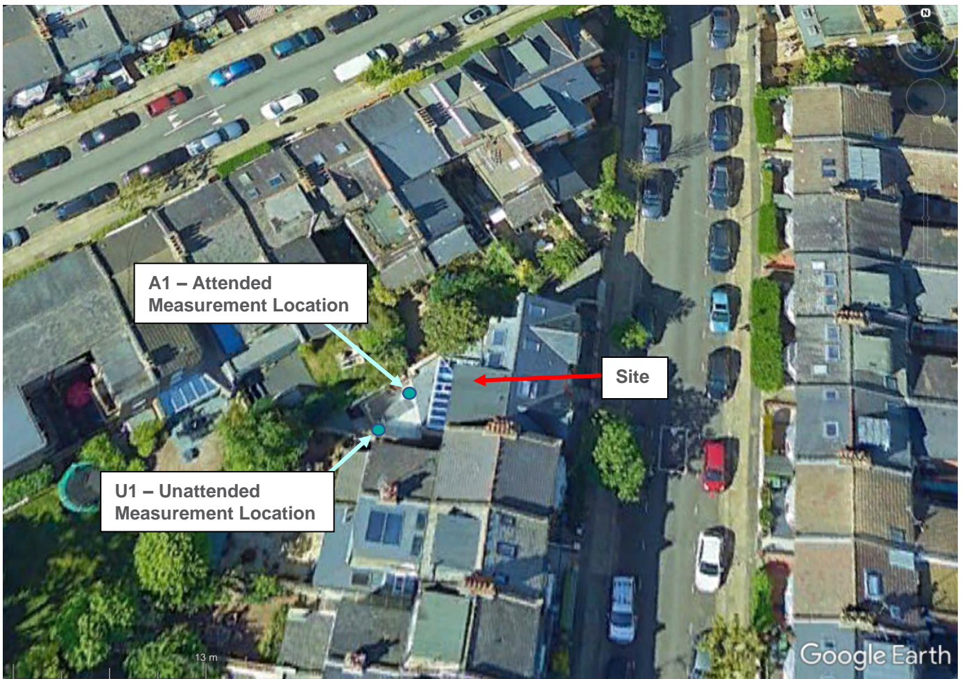
Figure 2 – Image showing proposed site noise monitoring location (Source: Google Earth™)
