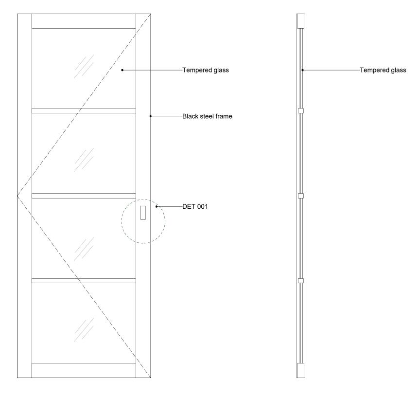
MODERN GLAZED DOOR- ELEVATION Scale: 1:10 MODERN GLAZED DOOR- SECTION Scale: 1:10 COPYRIGHT AND LIABILITY NOTES:
