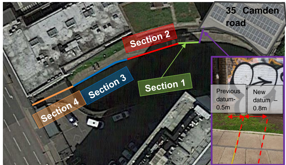
Figure 2.1: Wall Sections under consideration and Datum of Wall survey
