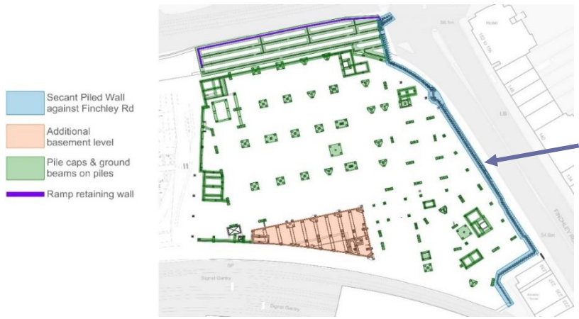
Figure 3 Existing O2 Basement Structure
