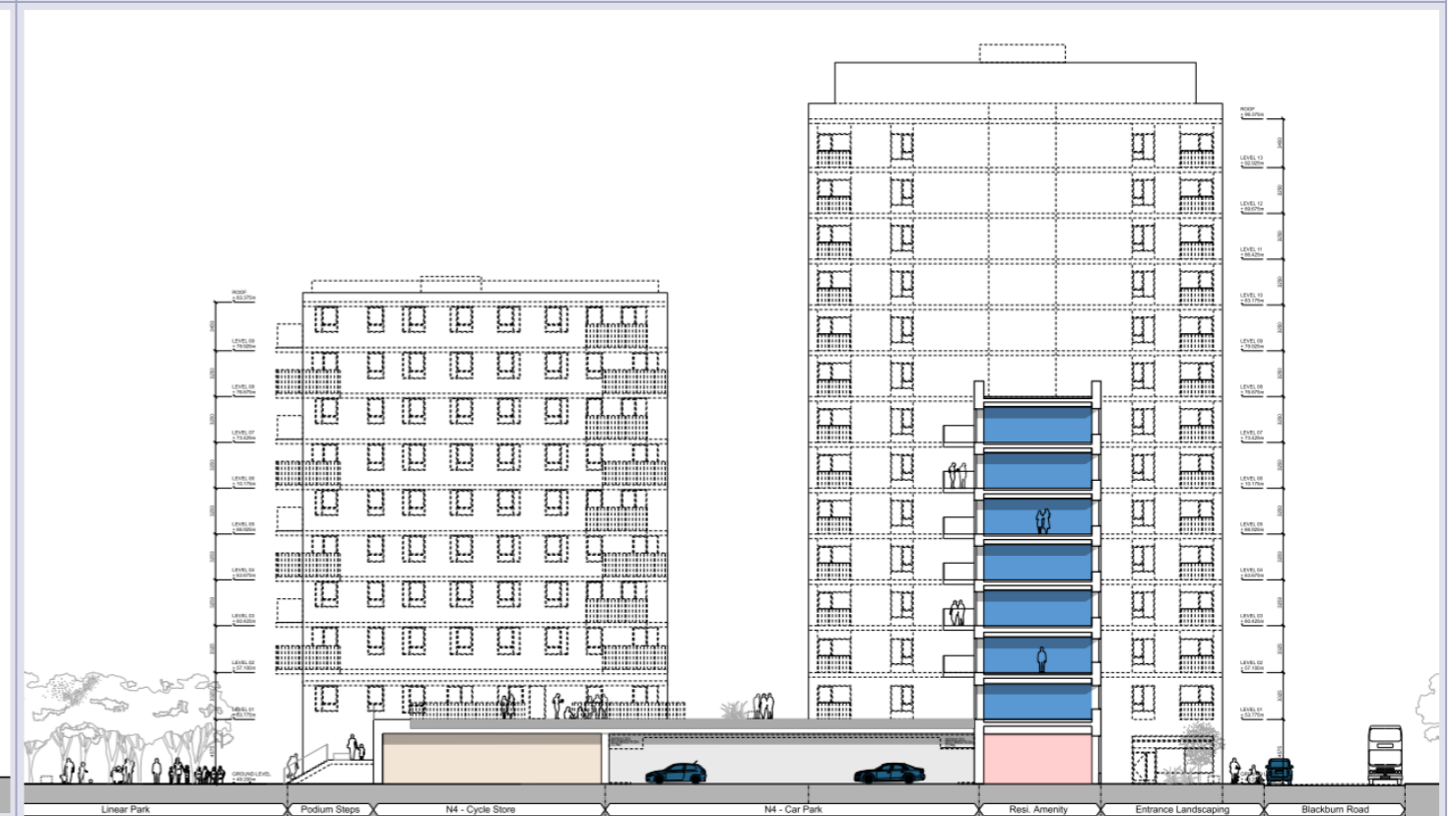
Cross section from east to north to south across N5, showing ground floor parking / bike storage, commercial / community space and refuse stores, with residential units on floors 0-14 and a raised podium garden on floor 1.
