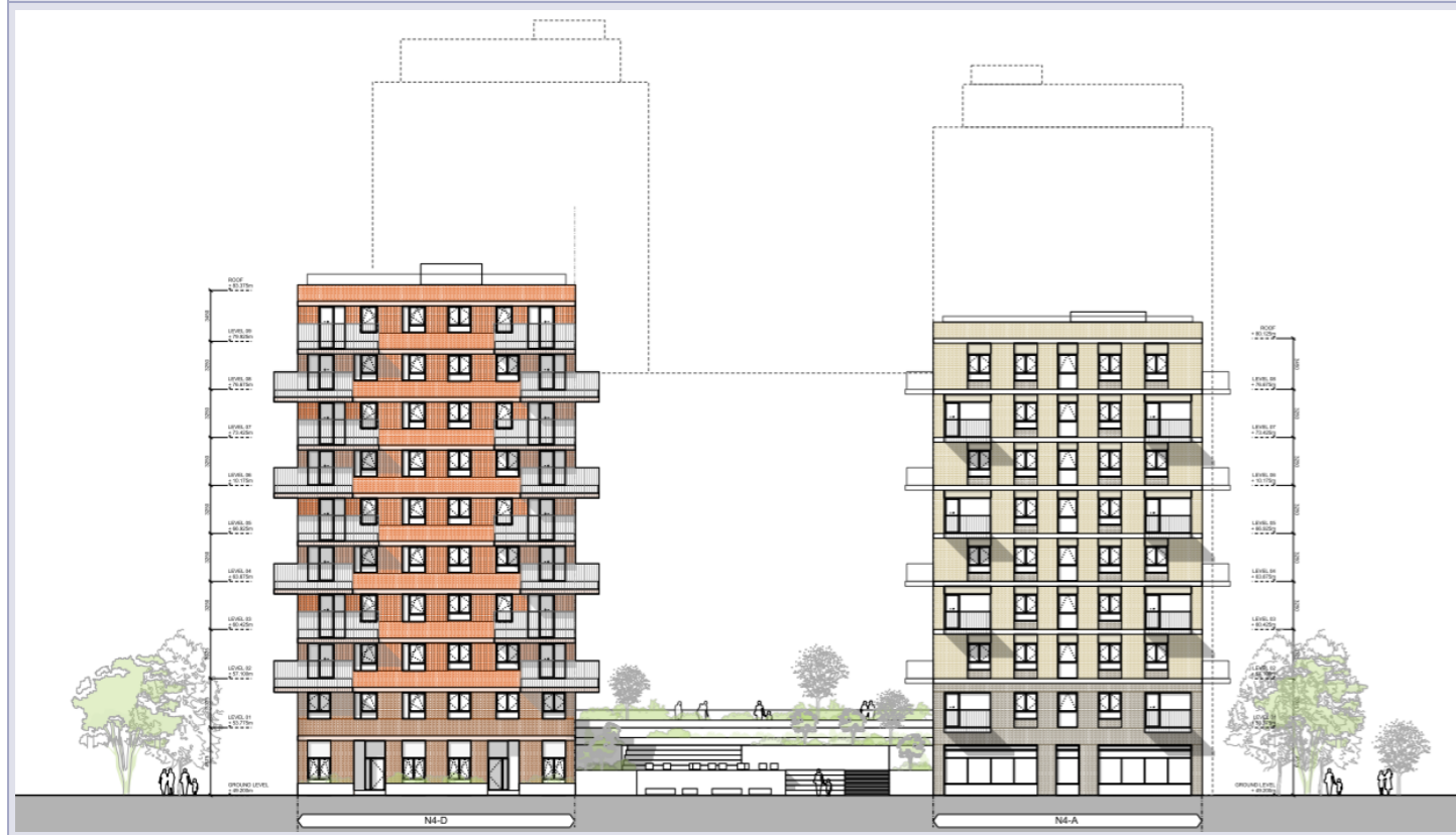
View of southern face of N4 development showing central raised podium gardens, with 8 & 9 story blocks in front and the outline of the 13 & 14 story blocks in the back.
