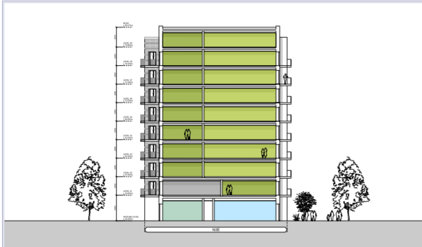
Cross section from east to west across N3, showing ground floor commercial / community space and bike & refuse stores, with residential units on floors 1-9.
