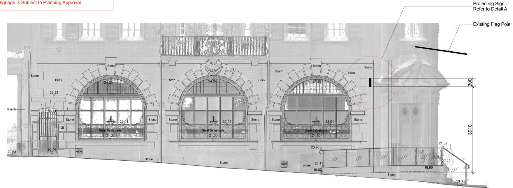
Powder coated –Aluminium Enclosure Finish: RAL 9011 1080 1000 -Affix to wall Line of Stone Entrance Arch Detail In front of proposed sign \_Internally Illuminated Lettering
