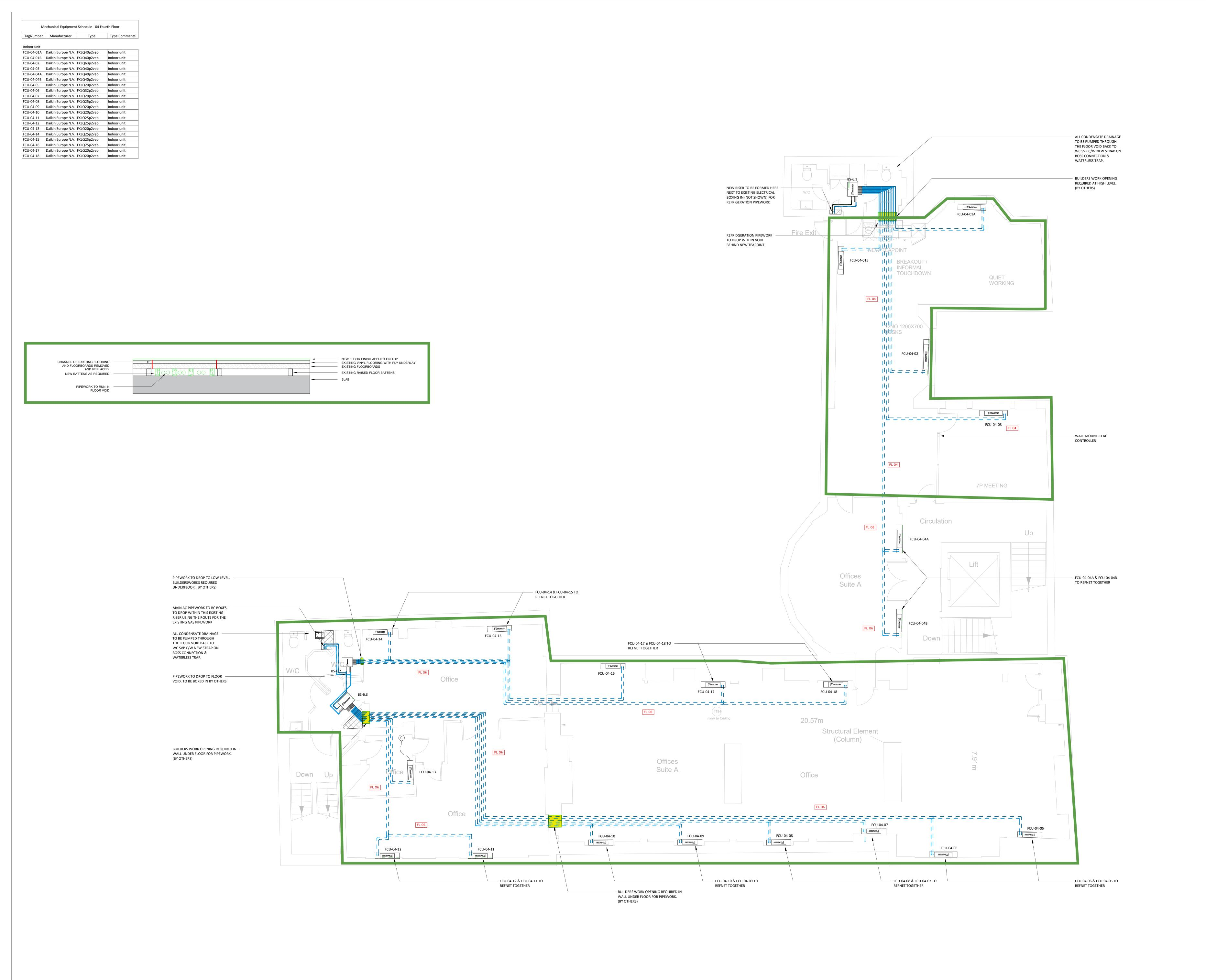
ALL CONDENSATE TO BE PUMPEDAND RUN WITH REFRIDGERATION PIPEWORK BACK TO SVP WITHIN WC BLOCK NO ALLOWANCE FOR MODIFICATIONS ON THE VENTILATION FOR THIS FLOOR. VENTILATION TO BE SURVEYED AND VALIDATED ONCE ON SITE AND ACCESSIBLE. LEGEND PIPEWORK AT LOW LEVEL TO BE BOXED IN (BY OTHERS) PIPEWORK AT HIGH LEVEL / WITHIN **CEILING VOID** — PIPEWORK WITH FLOOR VOID. POSSIBLE RISE LOCATION BUILDERS WORK OPENING IN WALL
