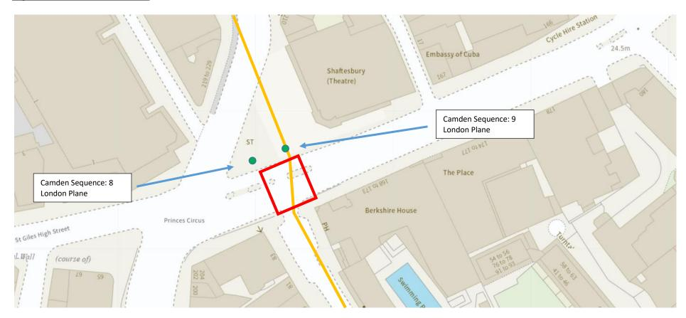
Trees to be affected by gas mains replacement works (including pre-enabling and trial holes) are highlighted below. This purely consists of severing roots to access the existing gas mains which are located within public highway. Above-ground works (ie. branch pruning) will not be required for these works.
