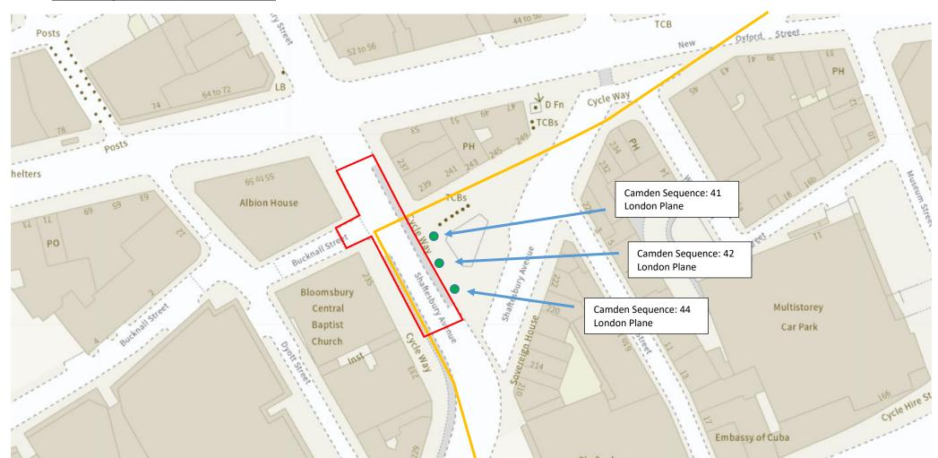
Trees to be affected by gas mains replacement works (including pre-enabling and trial holes) are highlighted below. This purely consists of severing roots to access the existing gas mains which are located within public highway. Above-ground works (ie. branch pruning) will not be required for these works.
