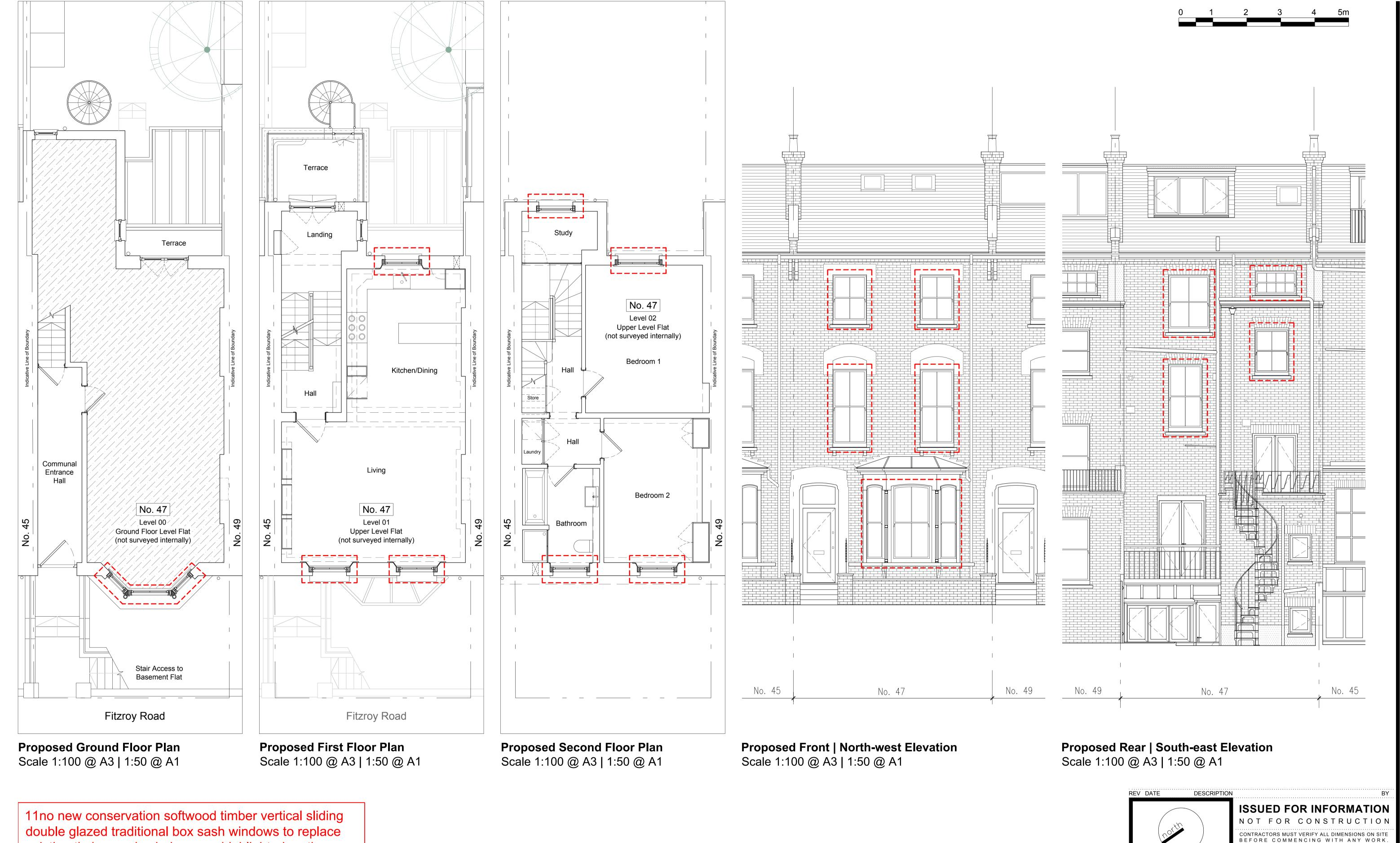
existing timber sash windows, as highlighted on the drawings above (including 7no new windows to front elevation and 4no new windows to rear elevation). All new windows to include integrated 22mm wide lambs tongue glazing bar with horns and to be painted white externally to match existing windows. 2no new sash lifts and 1no sash fastener to all new sash windows. Existing external window sills to be retained.
