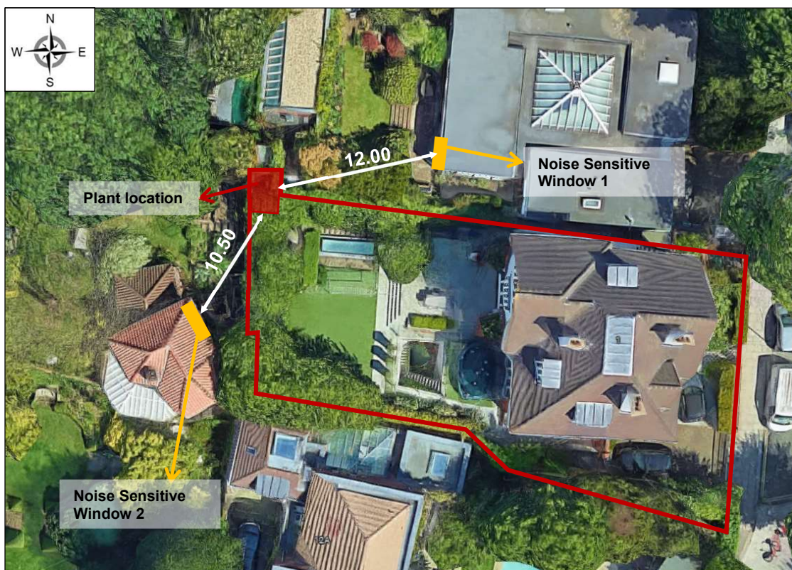
Proposed plant location plan (Imagery © 2022 Getmapping plc, Infoterra Ltd & Bluesky, Maxar Technologies, The GeoInformation Group, Map Data © 2022 Google)
