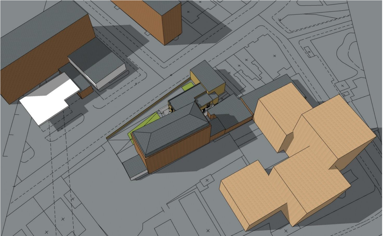
Fig 4. 3D model viewed from west. Shadows set to 12pm, 21st March (the equinox).
