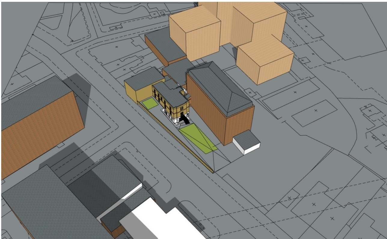
Fig 3. 3D model viewed from south. Shadows set to 12pm, 21st March (the equinox).
