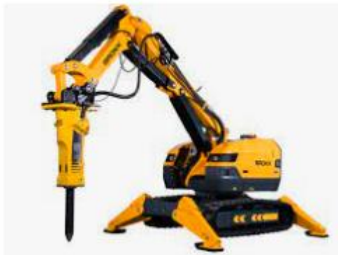
Brokk remote controlled demolition plant.
