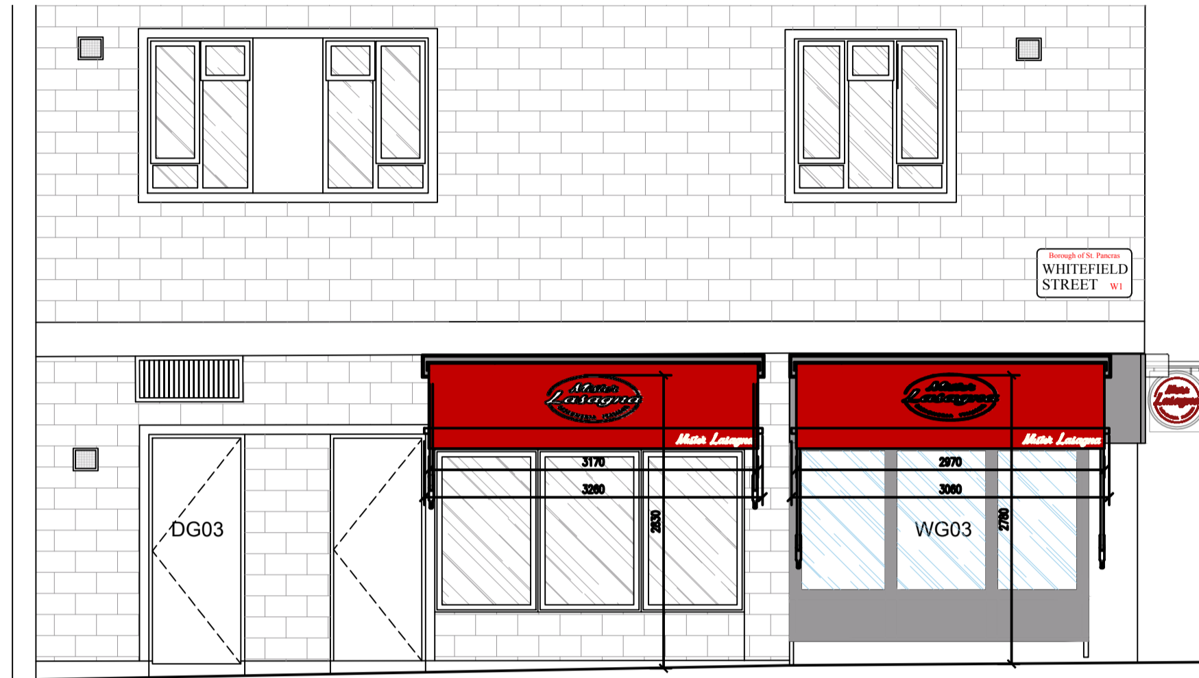
PROPOSED SIDE AWNINGS ELEVATIONS SCALE 1:50 @A1
