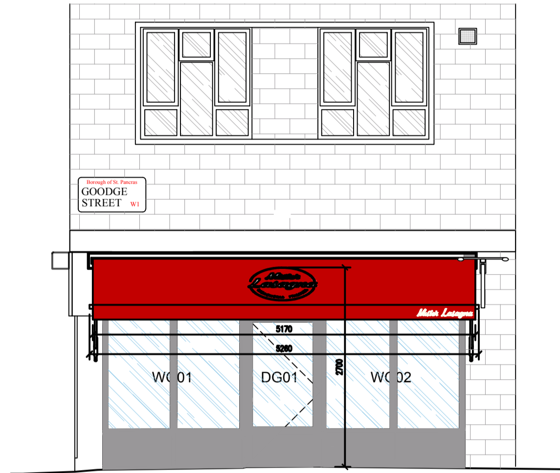
PROPOSED FRONT AWNING ELEVATION SCALE 1:50 @A1
