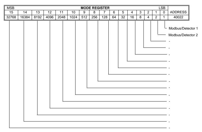
**Modbus/Detector Mode.** When this bit is set the relays will be connected to the Modbus register 40002. Relay 1 = bit 8, relay 2 = bit 9. When the bit is cleared then the relays will be connected to the detector.
