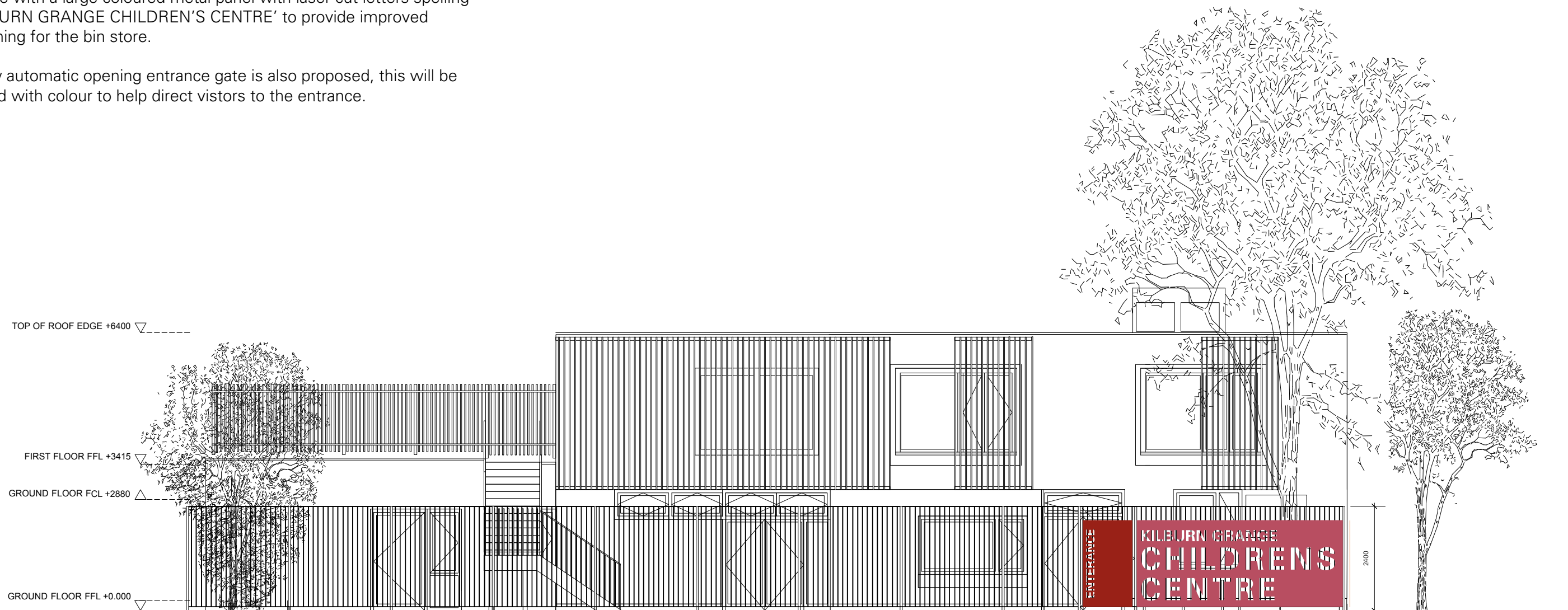
Proposed South elevation boundary fence - with new timber panelling secured to existing metal railings to increase height of perimeter to 2.4m
