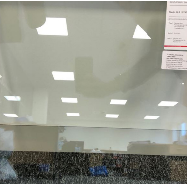
R6 - Glass Lower Material: Saint-Gobain glass, Pane 1; Diamant (4 mm) Annealed : Float PVB Standard (2 X 0,38 mm) Diamant (4 mm) Annealed : Float Cool-Lite Skn o83 Cavity; Argon (90%) / Air (10%) / 16 mm Pane 2; Diamant (4 mm) Annealed : Float PVB Standard (2 X 0,38 mm) Diamant (4 mm) Annealed : Float
