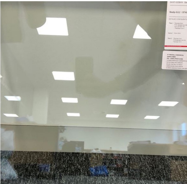
R7- Glass Upper Material: SunGuard SuperNeutral - SN 70/37, Pane 1; Guardian ExtraClear Glass, 4mm PVB Standard (2 X 0,38 mm) Guardian ExtraClear Glass, 4mm Cavity; Argon (90%) / Air (10%) / 20 mm Pane 2; Guardian ExtraClear Glass, 4mm PVB Standard (2 X 0,38 mm) Guardian ExtraClear Glass, 4mm
