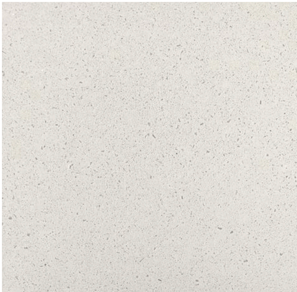
C2 - Concrete nodes Material: White precast concrete Supplier: Chiltern GRC Finish: Acid Etched
