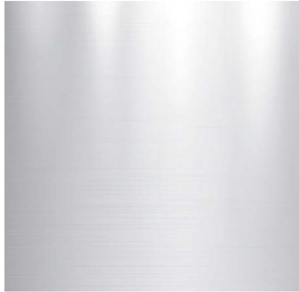
C5 - Recepton Window frames Material: Stainless steel Supplier: Rimex (fabricated by Stuctal/Rinaldi) Finish: Brushed - 240 grit
