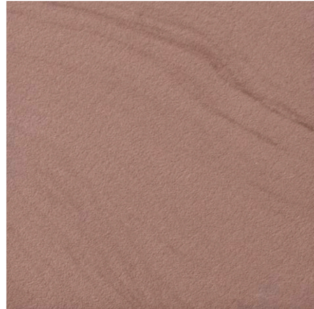
C1 - Stone cladding Material: Wuestenzell Red Sandstone Supplier: Hofmann Stone Finish: Aquapower
