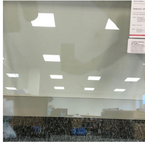
C6 - Glass Lower Material: Saint-Gobain glass, Pane 1; Diamant (6 mm) PVB Standard (2 X 0,38 mm) Diamant (6 mm) Cool-Lite Skn 076 Cavity; Argon (90%) / Air (10%) / 22 mm Pane 2; Diamant (5 mm) PVB Standard (2 X 0,38 mm) Diamant (5 mm)
