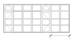
NOTE: bay windows are faceted and arranged along a curve, elevations show individual unfolded arrangement
