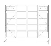
NOTE: bay windows are faceted and arranged along a curve, elevations show individual unfolded arrangement
