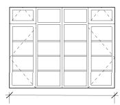
NOTE: bay windows are faceted and arranged along a curve, elevations show individual unfolded arrangement
