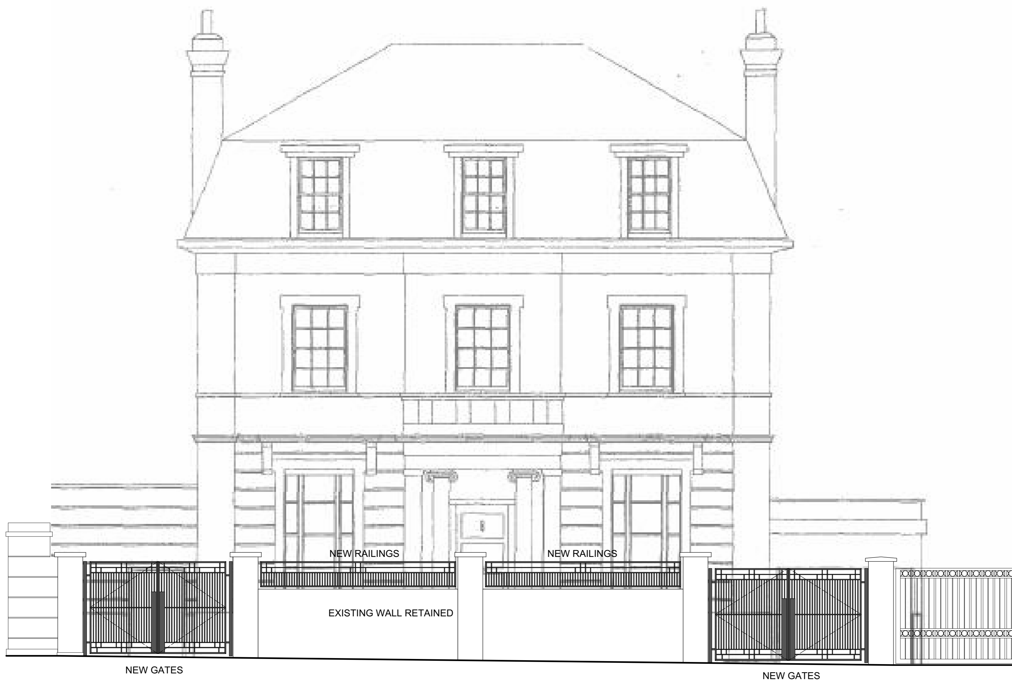
PROPOSED GATES AND RAILINGS FRONT ELEVATION
