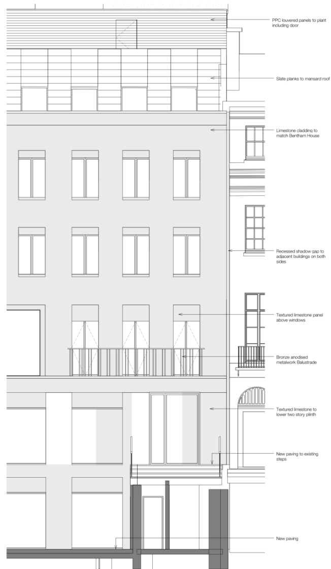
Left: Endsleigh Street elevation details Right: Section through new GS wing
