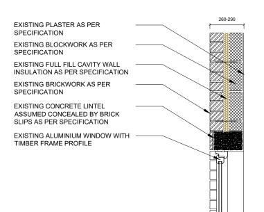
PURPLE PASSIVE VAPOUR CONTROL LAYER / AIRTIGHT FIBRE REINFORCED POLYMER EMULSION PASTE TO FORM CONTINUOUS SEAL WITH WINDOW MANUFACTURER EDPM PROPOSED 10MM EXTERNAL WALL AEROGEL INSULATION. RENDER FINISH AS PER SPECIFICATION WINDOW REVEALS AS PER EXTERNAL WALL FINISH.
