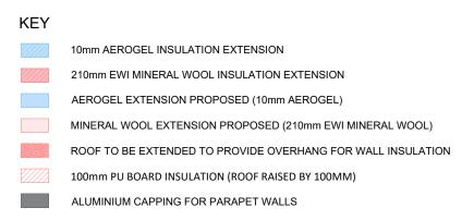
Note: All EWI insulation to be finished with brick slips to match the colour of existing brickwork (light brown / red) - See proposed finishes below from PermaRock's colour chart. Our preferred option would be the **Red Shadow**
