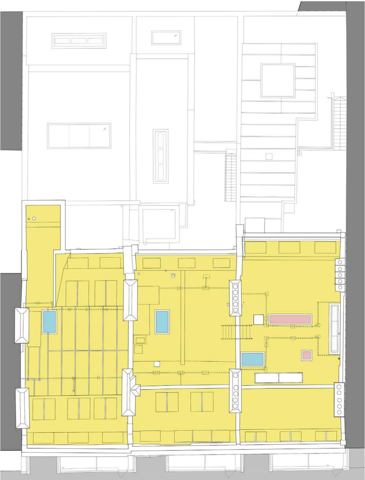
Proposed upper floor roof plan, colour coded to show proposals for repair/replacement
