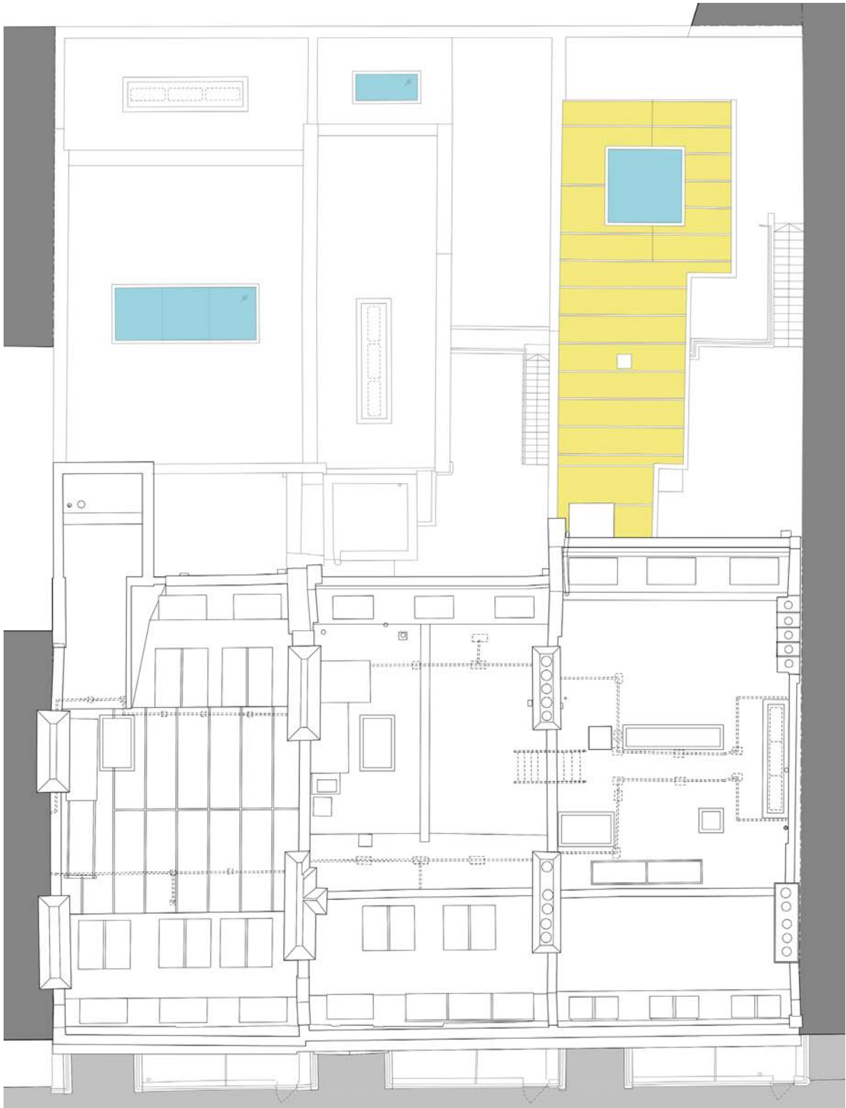
Proposed 1st floor roof plan, colour coded to show proposals for repair/replacement
