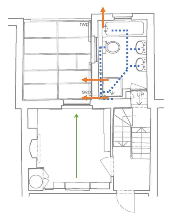
**EXTRACTION**: No change to extraction location. The existing opening on the side wall of the exterior is being used for the new bathroom extract and the new dryer extract.
