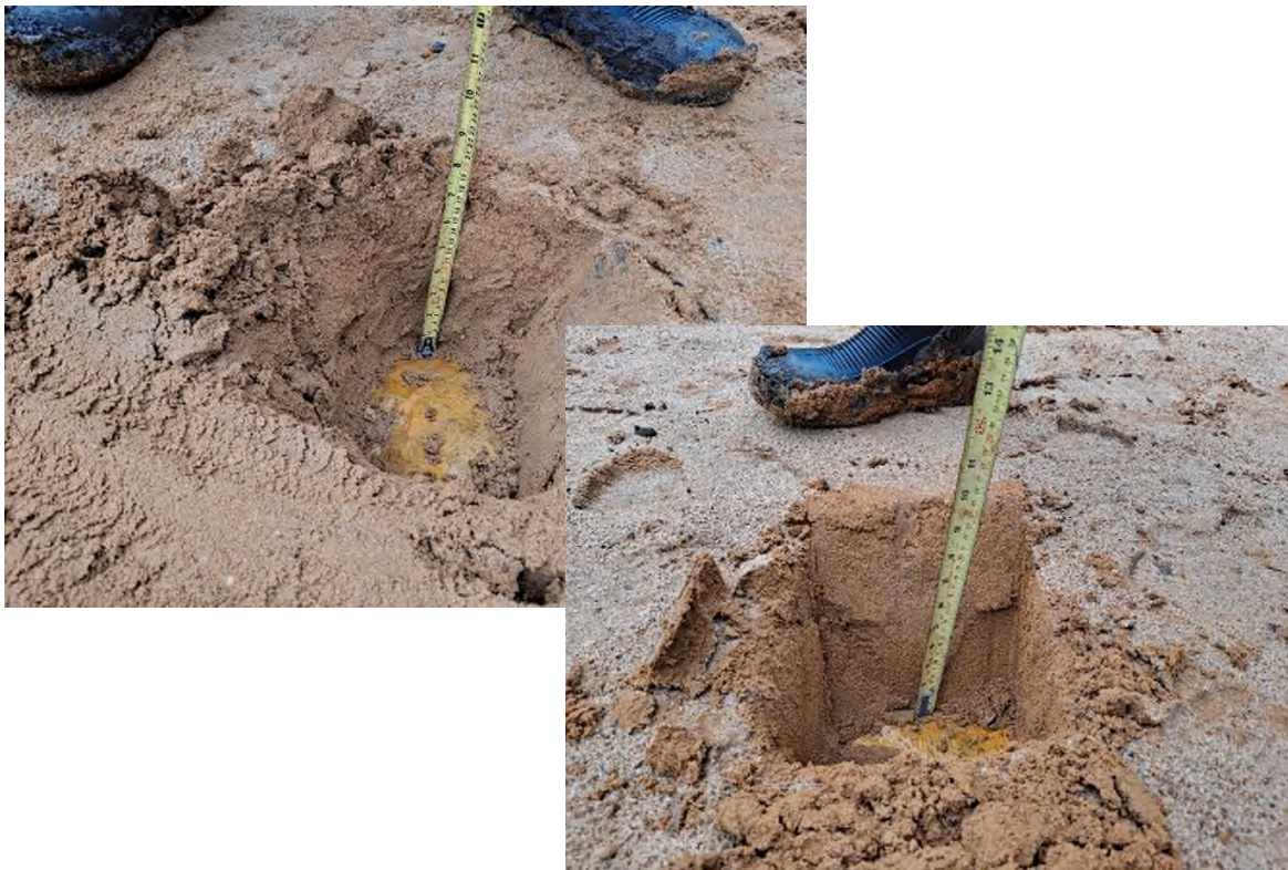
Plate 8: VISIT 15/02/22 – Thickness of subsoil in the location of former plots 25-28 (west of site)
