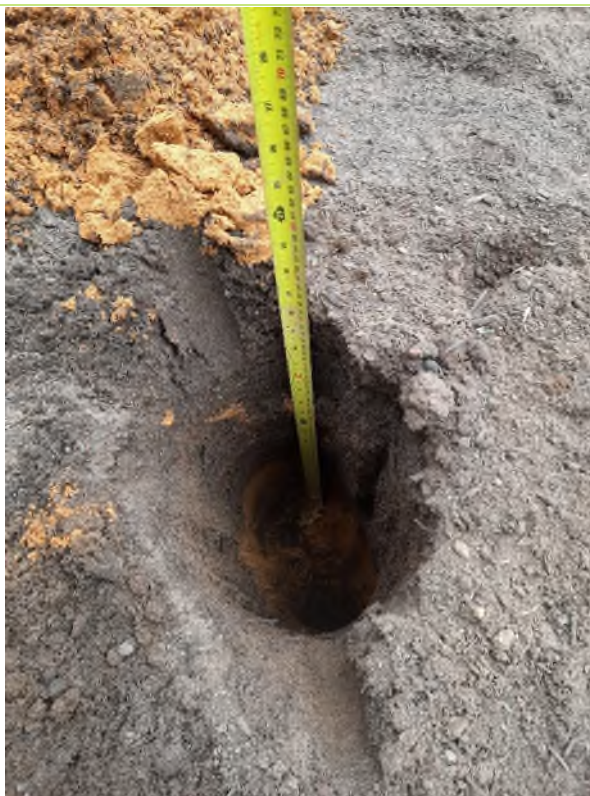
Plate 19: VISIT 05/04/22 – example inspection pit (plot 8b) showing 500mm cover
