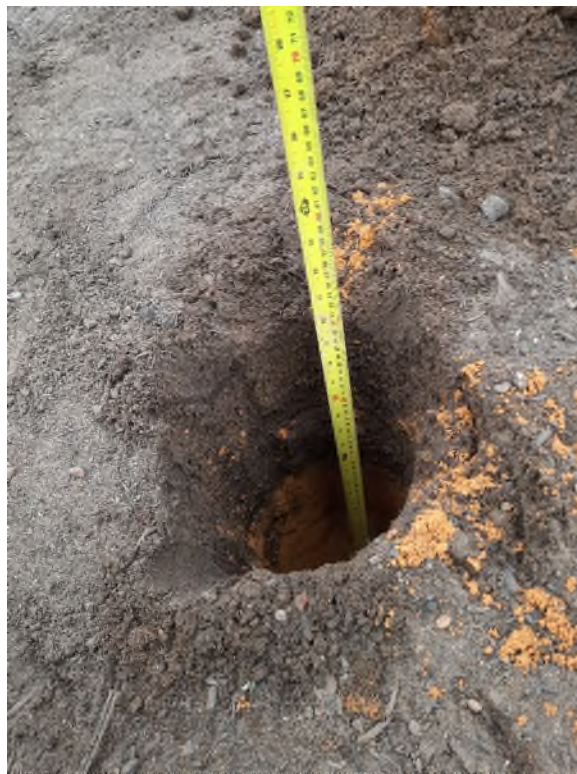
Plate 18: VISIT 05/04/22 – example inspection pit (plot 11a) showing 500mm cover
