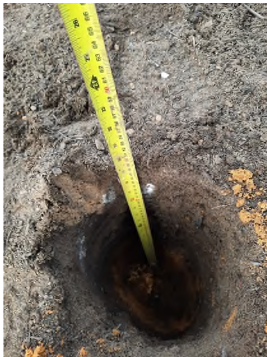
Plate 15: VISIT 05/04/22 – example inspection pit (Plot 1) showing 500mm cover
