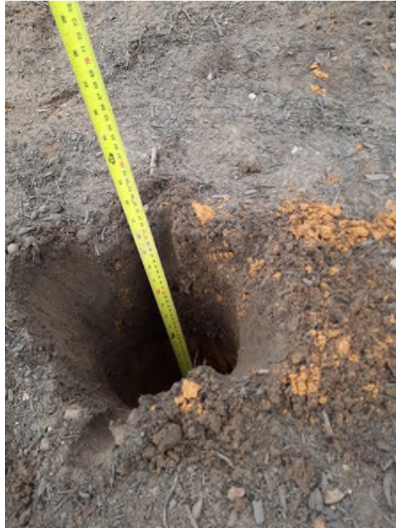
Plate 17: VISIT 05/04/22 – example inspection pit (plot 15b) showing 500mm cover
