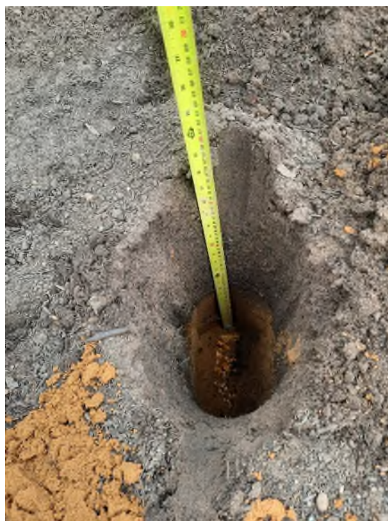
Plate 16: VISIT 05/04/22 – example inspection pit (plot 16a) showing 500mm cover
