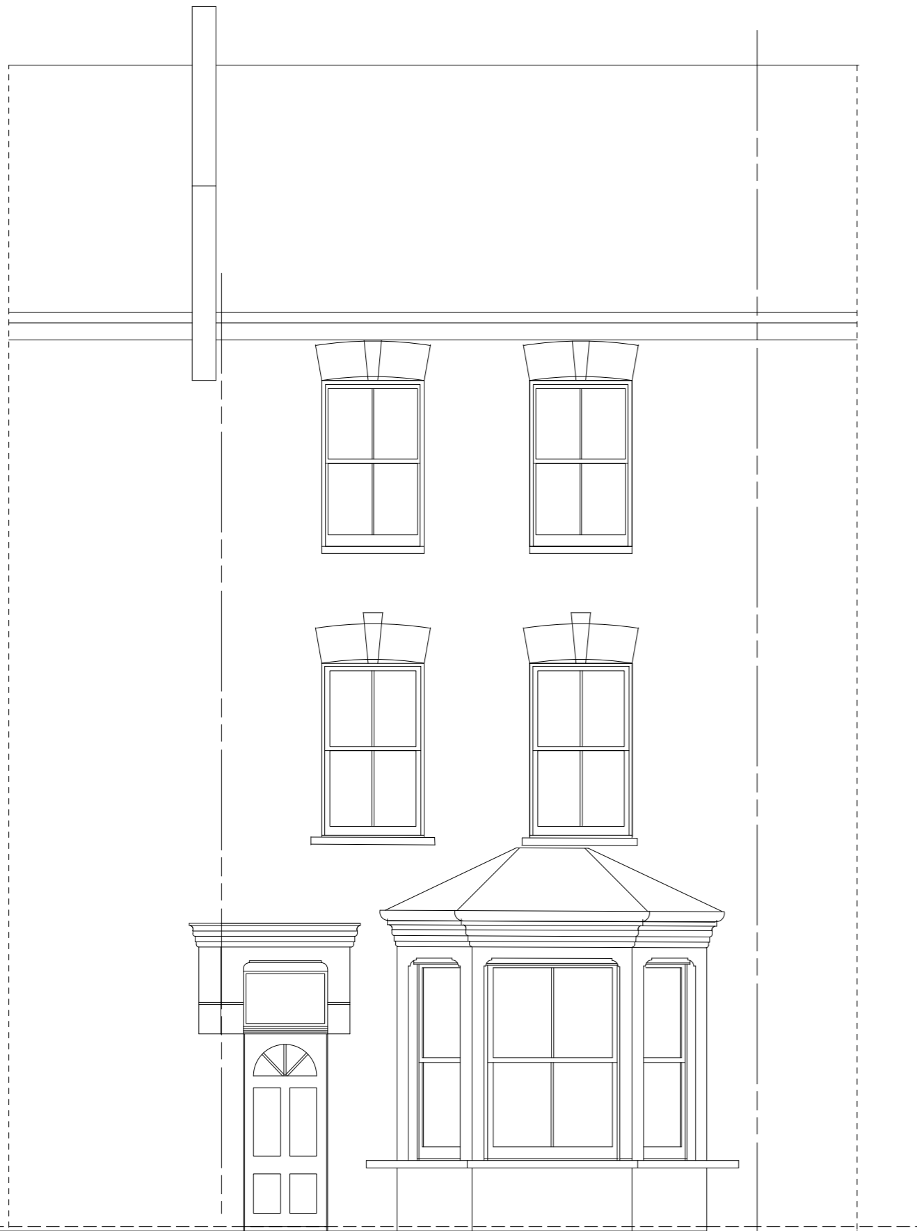
FRONT ELEVATION AS EXISTING
