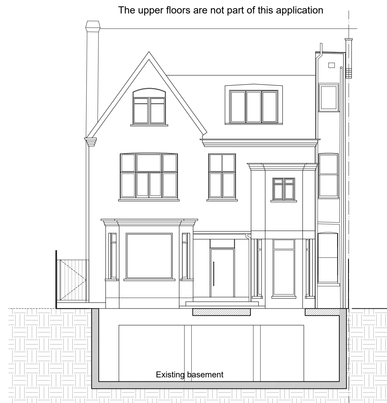
Existing Front Elevation/Section through front lightwell Scale 1:100
