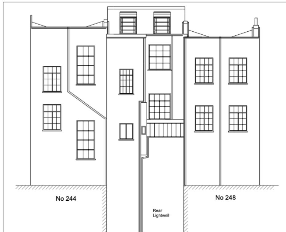
Figure 15: Proposed rear elevation showing mansard roof extension with dormer windows and addition to outshoot.
