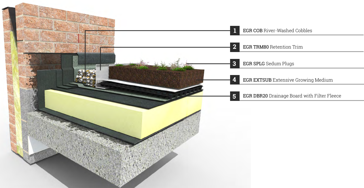
The diagram is for illustration only. The waterproofing membrane demonstrates just one example of applicable detailing. The protection layer above the waterproofing is the responsibility of the waterproofing membrane manufacturer unless specified.
