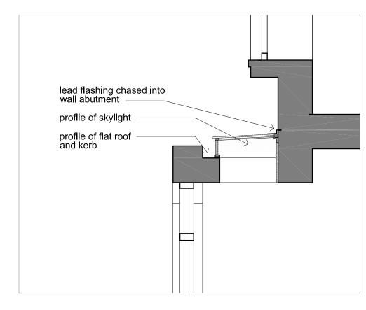
SECTION THROUGH SKYLIGHT AT 1:20 SCALE
