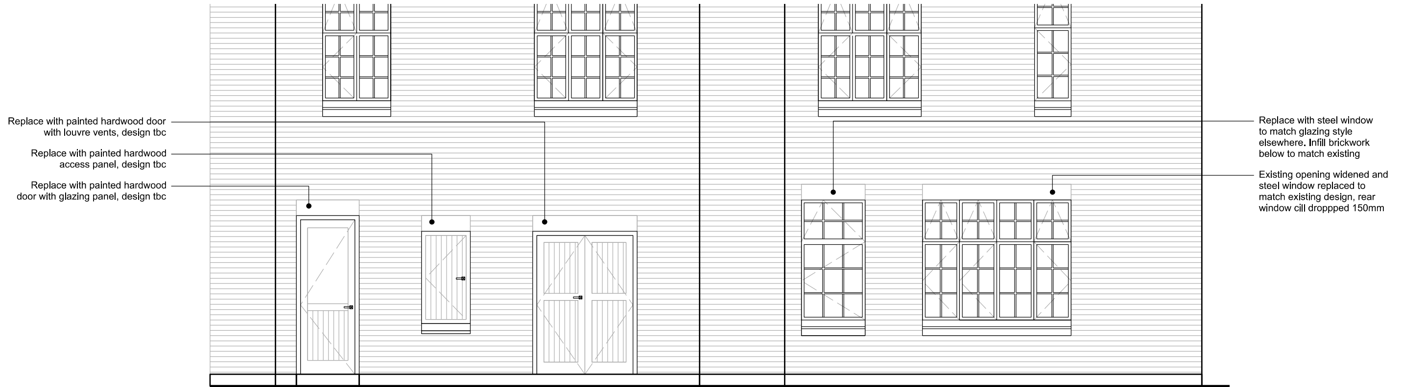
↑ Drawing of proposed new doors. To be high-performance hardwood doors, painted white, with brushed stainless steel ironmongery
