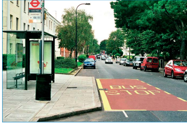
Bus boarder in Belsize Road
