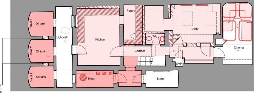
Historic openings between J vaults to be reinstated with modern infill brick removed
